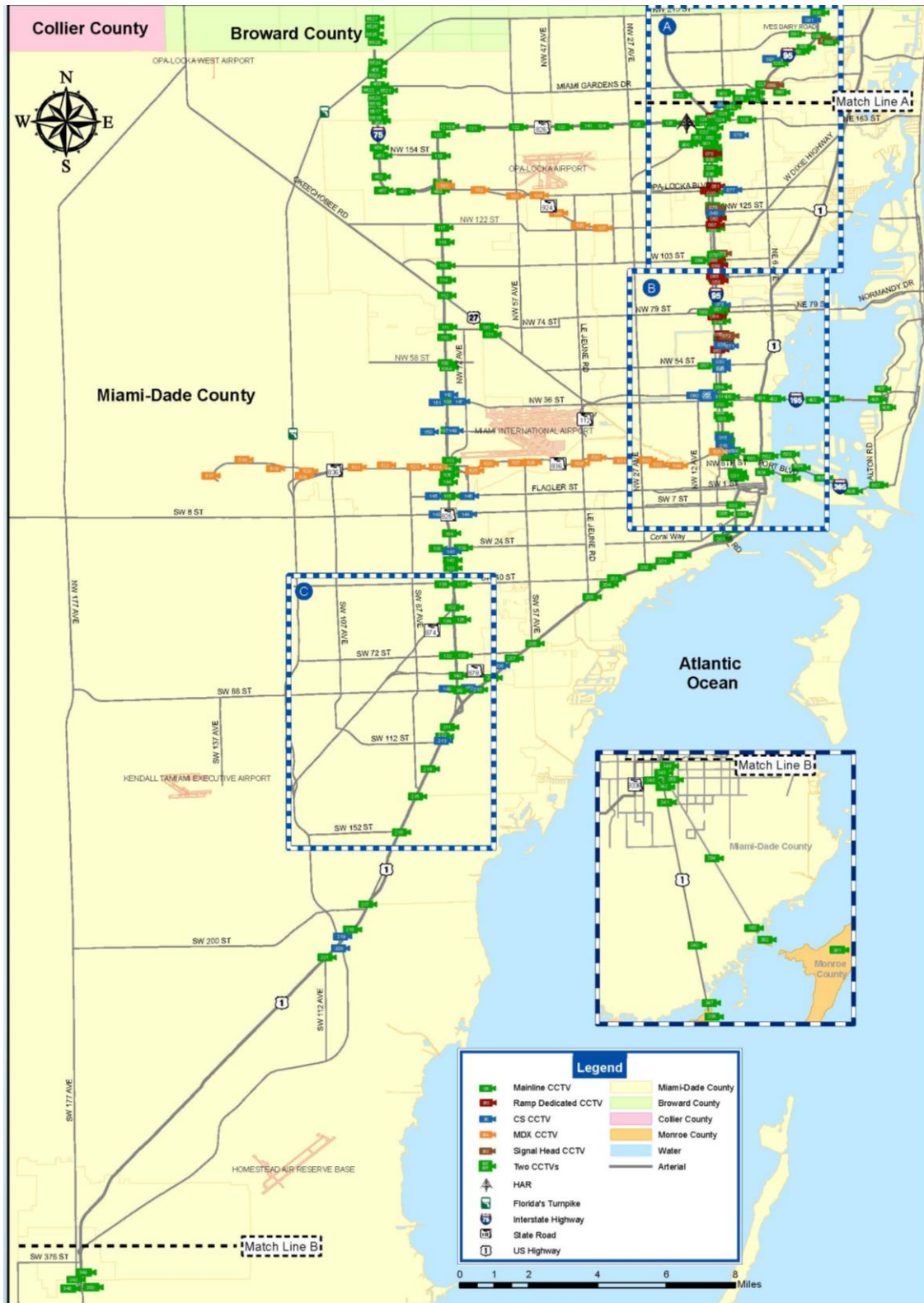
FIGURE 3 LOCATIONS OF FDOT D6 TMC ITS DEVICES - CCTVS
